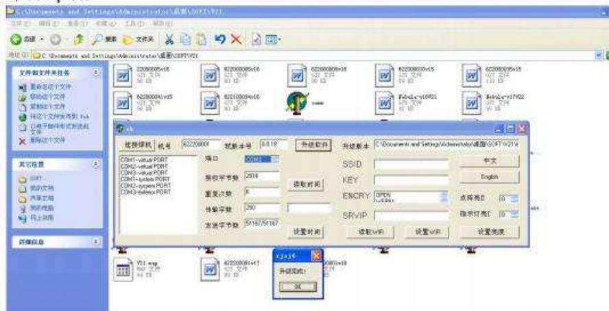
If there's something wrong with connecting to the welding machine, the reasons may be following: 1. Disconnection or short circuit of the cable, two 485 cables are in reverse order, please check the cables carefully. 2. Something wrong with the USB-RS485 converter, suggest the UT-850 or
