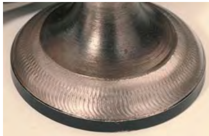
Smooth surface and spatter free Coating.
