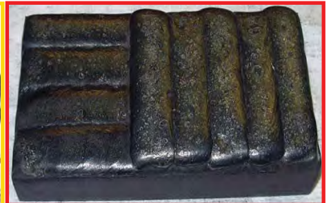
DO 390 can be built up to a thickness of up to 12.5mm (1/2 inch)
