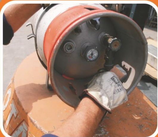
Wear gloves when connecting hose to avoid cold burns
