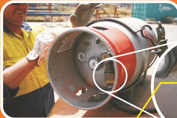
Hose connection must be tightened all the way to the top
