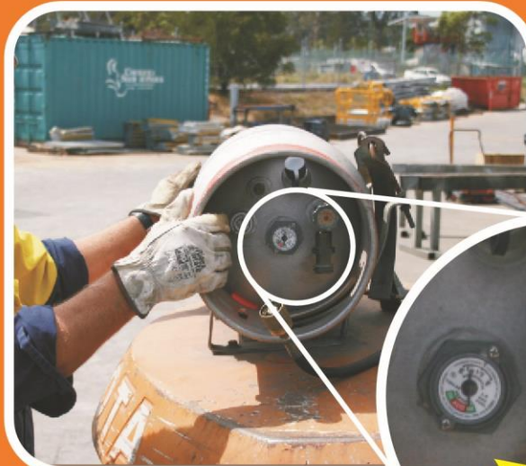
Make sure connection is vertical to ensure all gas is used
